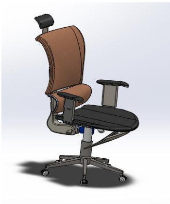
Figure 3. Design chair in 3D side view [designed by solidworks 2017 x64 edition].
