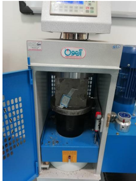
Figure 7. Performing compressive strength test of concrete.
