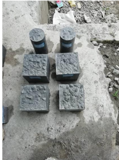
Figure 3. Construction of a control sample.
