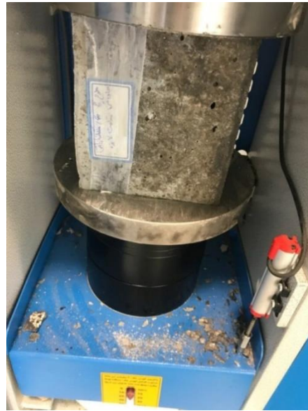
Figure 5. An example of concrete with rice husk ash containing recycled aggregate.
