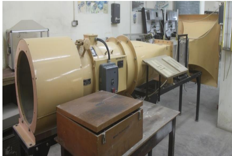
Fig. 1. Analogue PLINT & partners subsonic wind tunnel machine.
