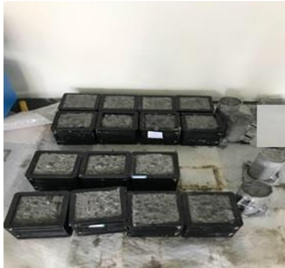
Figure. 4. Sample construction with rice husk ash and microsilica.
