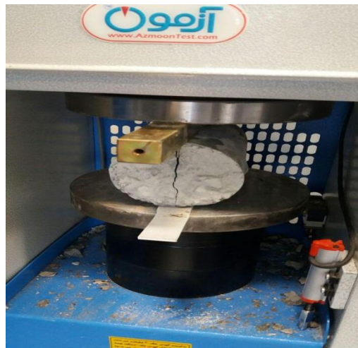
Figure. 8. Performing compressive strength test of concrete.
