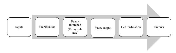
Figure 1. Structure of FMEA Based on Fuzzy Theory.
