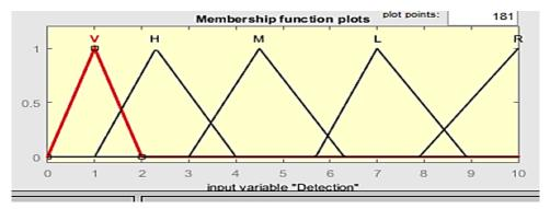
Figure 4. Membership Function for Detection (Matlab).
