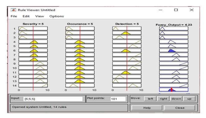
Figure 7. Inputs and Output Views of Risk Priority in Matlab.
